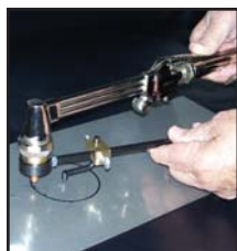
16229 Adjustable Circle Cutting Guide Cutting range from 5/8" - 12" holes
